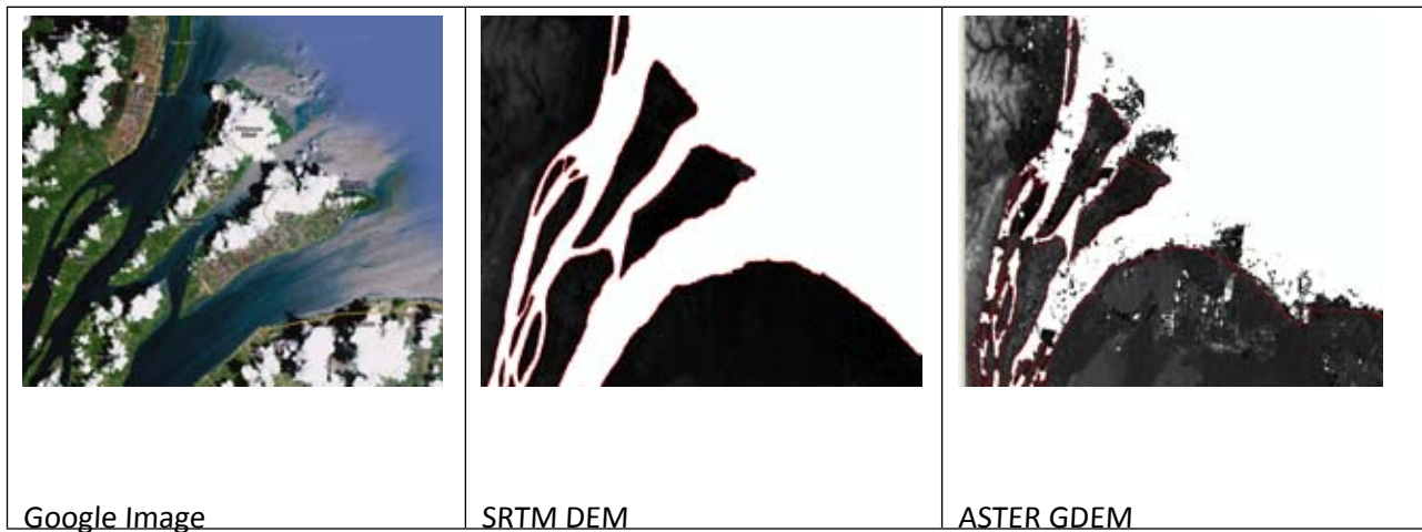
Figure 21: Comparison of SRTM DEM and ASTER GDEM Data with Google maps image for reference
